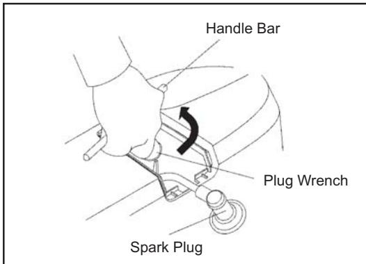
5. Visually inspect the spark plug. Discard it if the insulator is cracked or chipped. Clean the spark plug with a wire brush if it is to be reused.
