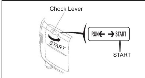
Do not use the choke when the engine is warm or the air temperature is high.
