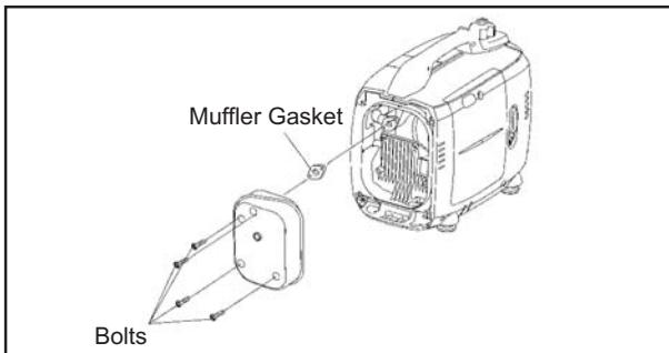
3. Check the muffler gasket replace if damaged. Reinstall the muffler gasket, the muffler and the muffler protector in the reverse order of removal.
